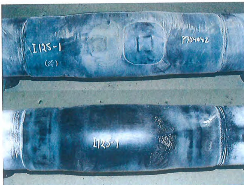
Picture 4 Joint I125-1 upper side (a) and under side (b) after sand box test.
